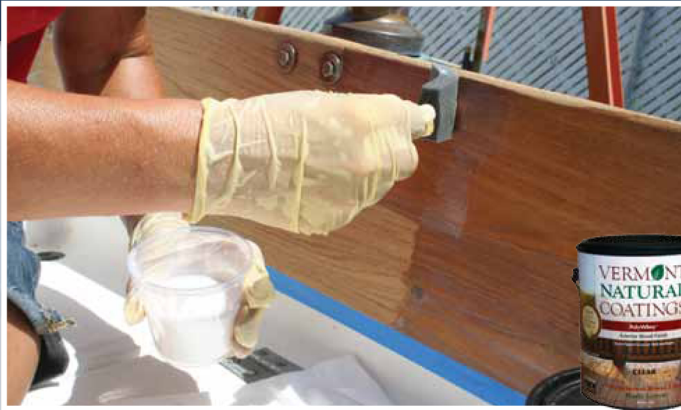
In a comparative field test, PS applied Vermont Natural Coatings PolyWhey and Interlux Cetol Natural to the teak aboard one of our test boats.
